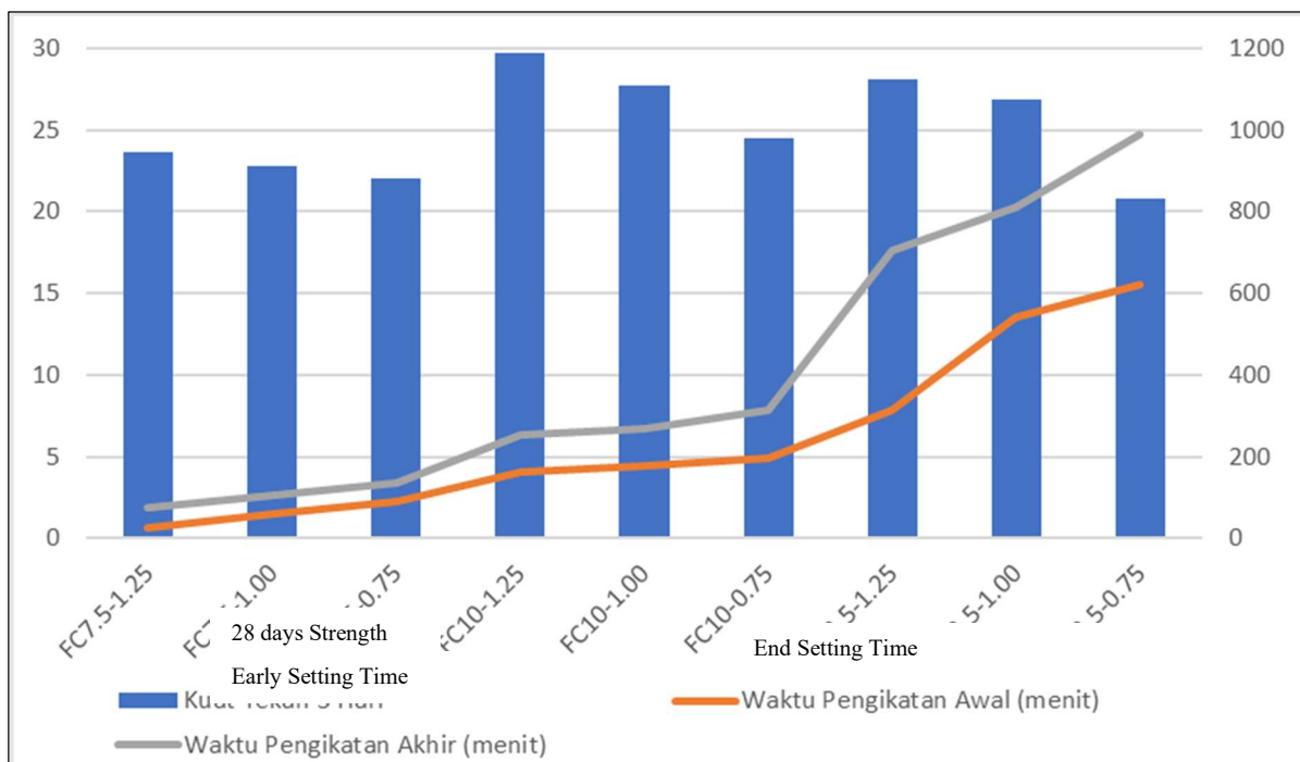
Figure 10. Relationship between setting time and compressive strength of geopolymer paste on day 28
