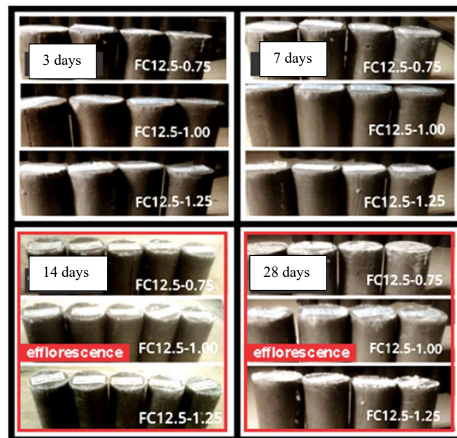
Figure 7. Visual Observation of specimens at ages 3, 7, 14, and 28 days
