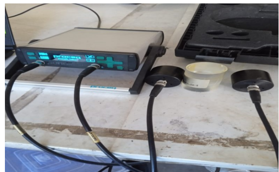
Gambar 2. Kalibrasi Ultrasonic Pulse Velocity (UPV)
