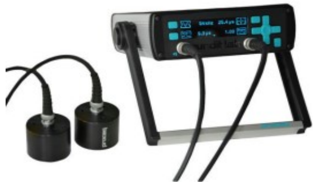
Gambar 1. Ultrasonic Pulse Velocity (UPV) [11]
