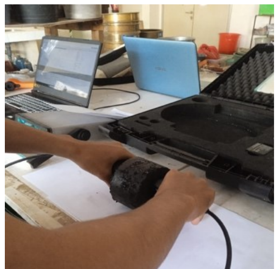
Gambar 3. Pengujian Ultrasonic Pulse Velocity (UPV)
